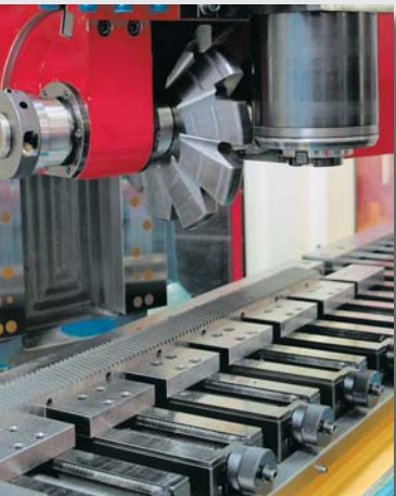
2 Hydraulic clamping fixture, adjustable from 1 to 225 mm (360 mm)
